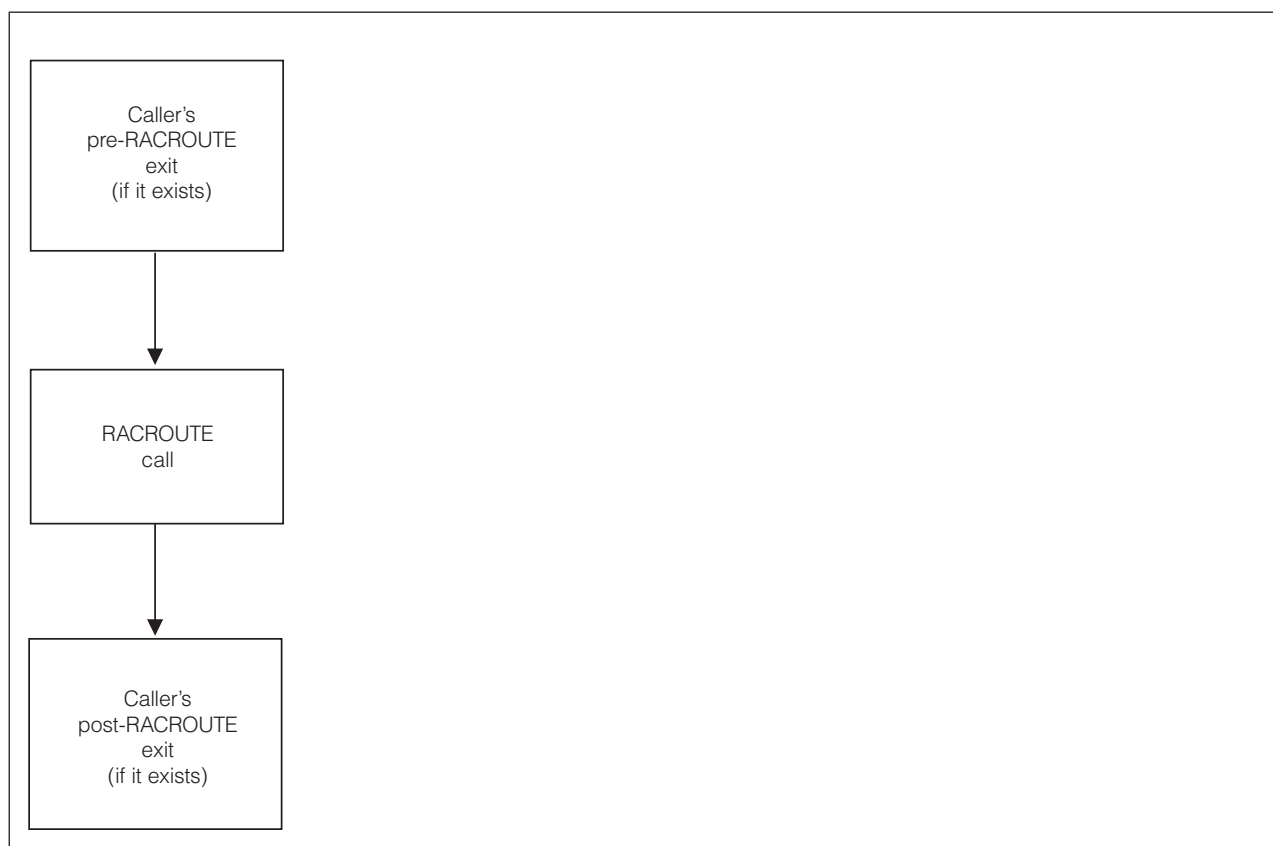
Figure 64. Process flow of callers of RACF for RACROUTE REQUEST=AUTH requests
